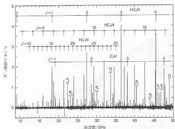
**Figure 1.** A compressed atlas of the 8.8-50 GHz spectrum toward TMC-1 (cyanopolyne peak). The abscissa is the frequency in GHz, and the ordinate is the line intensity expressed in the temperature scale.
